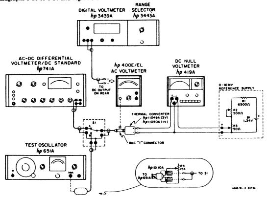
Figure 5-1. Accuracy and Frequency Response Test Setup
