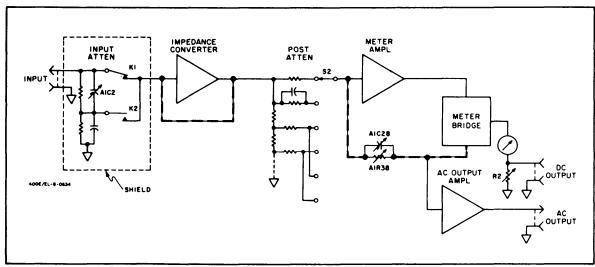
Figure 4-1. Simplified Block Diagram
