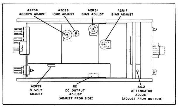
Figure 5-3. Location of Internal Adjustments
