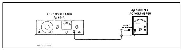
Figure 5-2. Input Impedance Check
