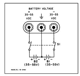
Figure 3-2. External Battery Connection
