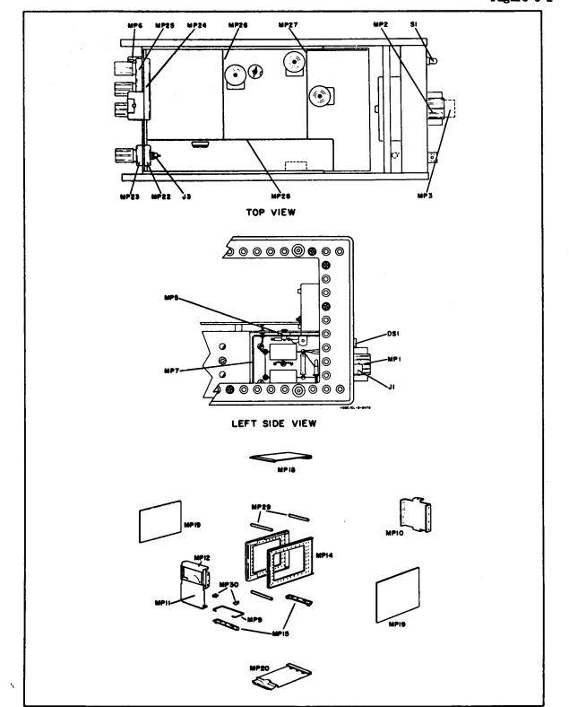
Figure 6-2-Location of Important Mechanical Parts
